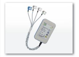
In connection with the MIPM MRI ECG pad the digital artifact filter ensures reliable ECG readings during the full course of a scanning procedure, even during strong gradient scanning sequences.
