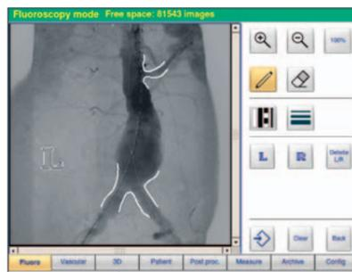
**AMT:** The Anatomical Marking Tool (AMT) enables the user to apply markings and left / right labels to live images using the touchscreen. It is also a straightforward tool to mark blood vessels branches or implant positions on live images.
